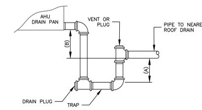
AHU CONDENSATE DRAIN DETAIL NTS
