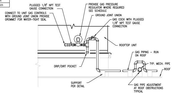
ROOFTOP UNIT GAS PIPING DETAIL NTS
