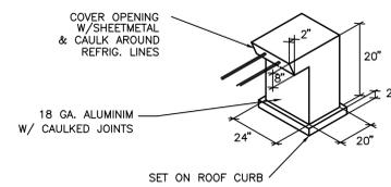
REFRIG. LINE THRU ROOF DETAIL NTS
