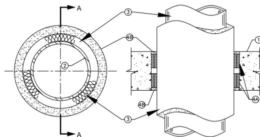
1. **Floor or Wall Assembly** - Min 5-1/2 in. thick reinforced lightweight or normal weight (100-150 pcf) concrete. Wall may also be constructed of any UL Classified **Concrete Blocks\***. Diam of opening to be 1 in. to 1-1/4 in. larger than outside diam of insulated pipe. Max diam of opening is 18 in.
