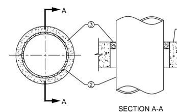
1. **Floor or Wall Assembly** - Min 4-1/2 in. thick lightweight or normal weight (100-150 pcf) concrete. Wall may also be constructed of any UL Classified **Concrete Blocks\***. Max diam of through opening is 12-1/4 in.
