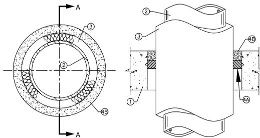
1. **Floor or Wall Assembly** - Min 2-1/2 in. thick reinforced lightweight or normal weight (100-150 pcf) concrete. Wall may also be constructed of any UL Classified **Concrete Blocks\***. Max diam of opening is 18 in.
